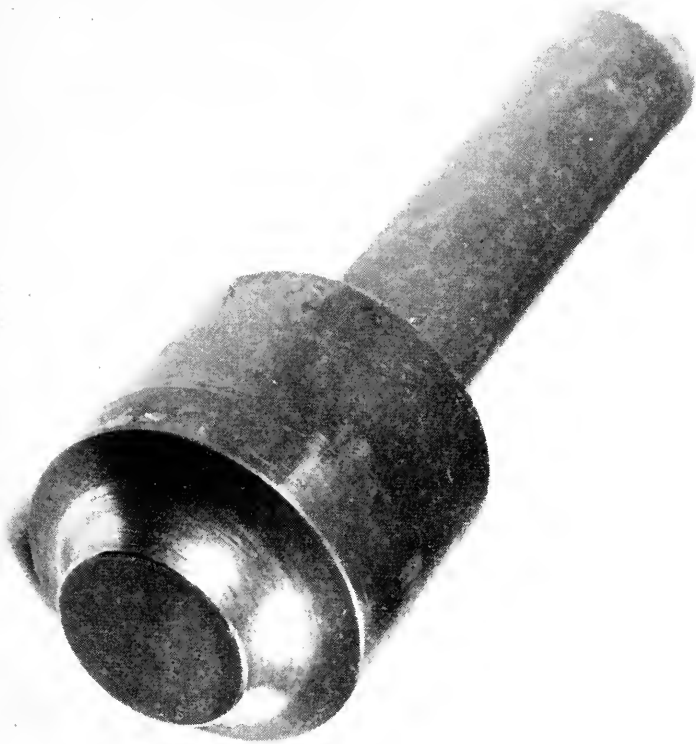
Fig. 17—Tool for peening edge of bolt hole.
